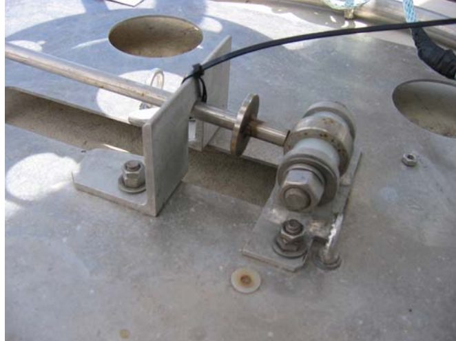
Figure 19. Prototype I Acoustic Release Anchor Point. The lever arm was designed to decrease the load on the burn wire.
