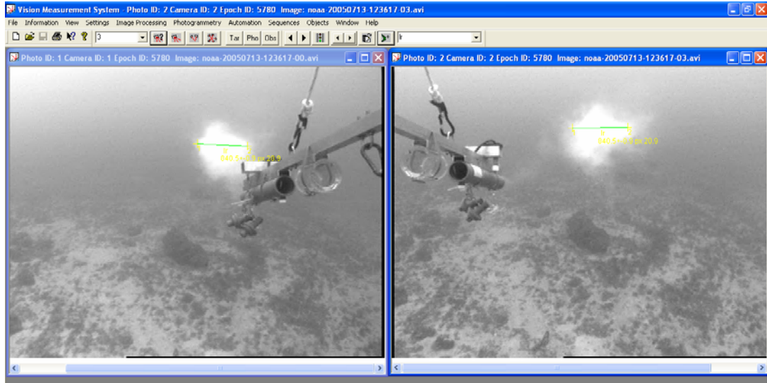
Figure 53. Bait Dispersal Measurement. The bait cloud is measured as it moves away with the current. The bait cloud is enhanced by using flourescene dye.
