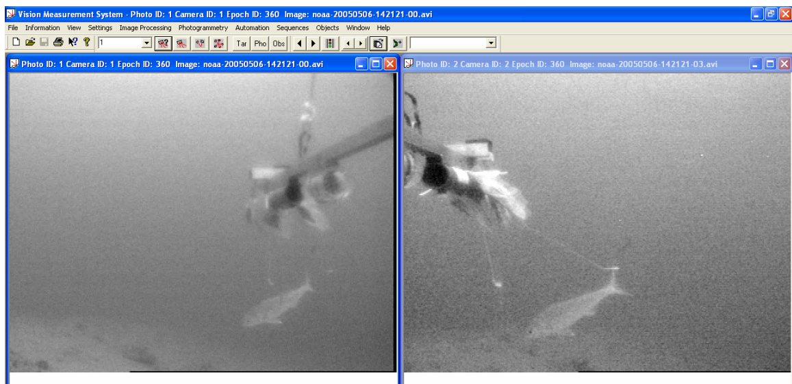
Figure 42. Frame grab of video imported into VMS software. The left image was collected using the ROS Navigator camera, the right image using the Watec camera.
