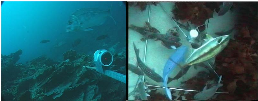
Figure 15. Left image horizontal looking bait station (courtesy of Harvey). Right Image downward looking bait station (courtesy of Timothy Langlois).
