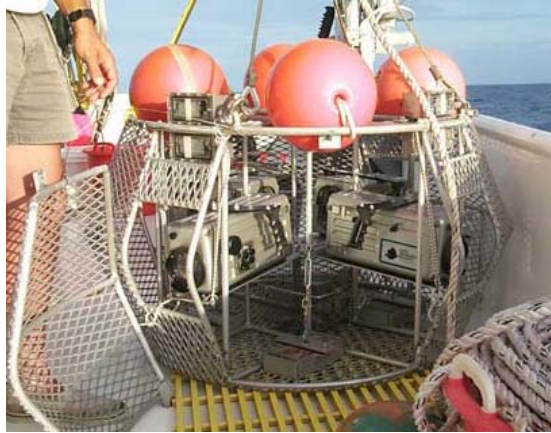
Figure 2. Baited Camera System Used by Gledhill et al (Southeast Fisheries Science Center) in the Gulf of Mexico.
