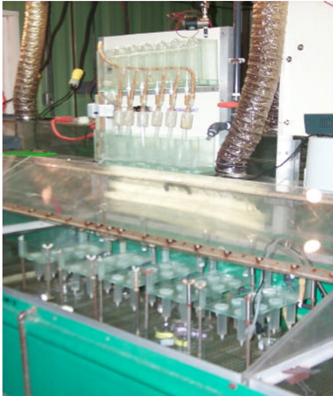
Photo 3. 250-ml beakers in an intermittent flow diluter system; 7 additional water every day.
