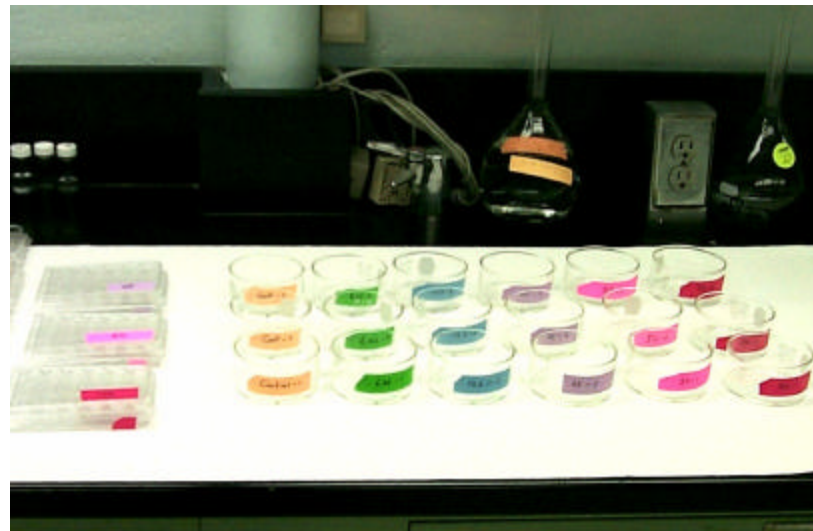
Photo 2. 24-well polystyrene tissue-culture plates and 200-ml crystallizing dishes.
