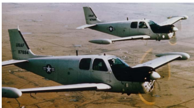
The QU-22B could be visibly distinguished from the earlier "A" models by the large generator positioned above the engine giving the aircraft a noticeable hump.
