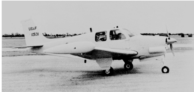
The YQU-22A's generator and tip tanks are visible in this photograph. The lack of de-icing equipment is also apparent.
