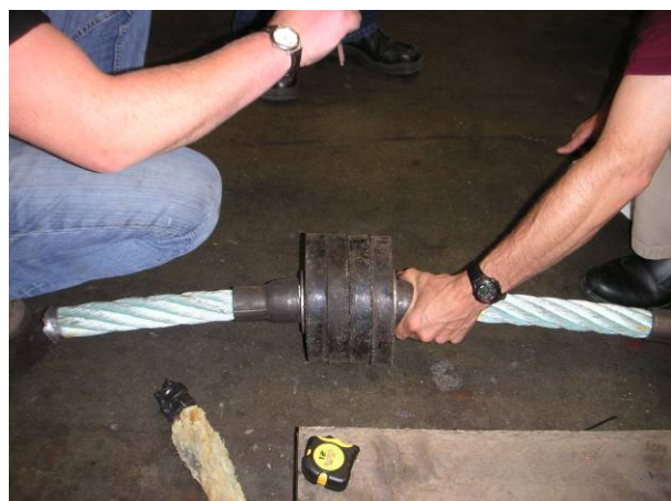
8 inch elevating discs mounted on body of 2-inch (52-mm) combination wire with stopper swages each side.
