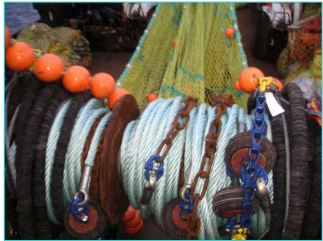
Sweeps and bobbins wound on the forward net reel once the net is unwound
