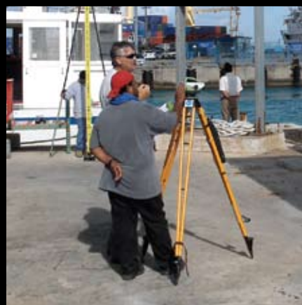
(Facing page) PSC staff assisted with field tests in Samoa for the NGS Shallow Water Positioning System (SWaPS). This new system provides precise horizontal positions for visible underwater features. Imagery is recorded and entered into a GIS, where data can be viewed, archived, and monitored for changes.
