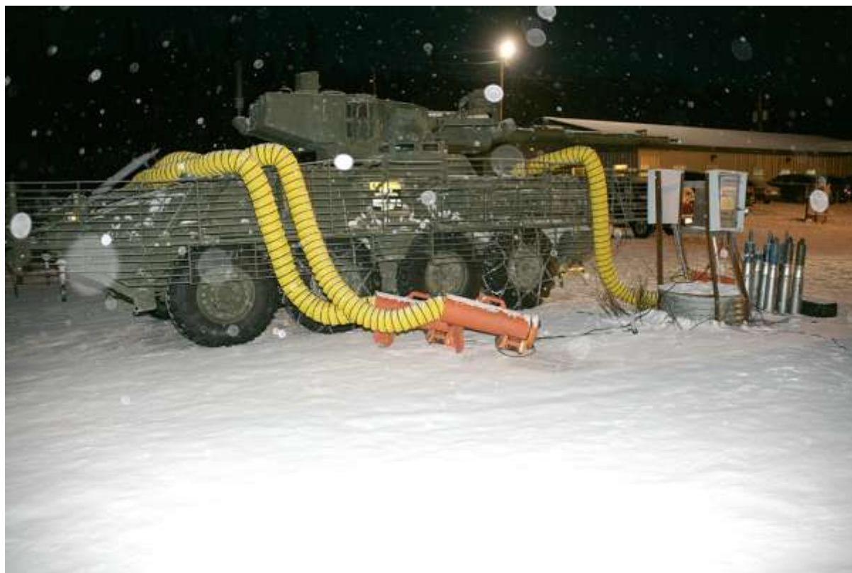
Figure 2.1 Test Vehicle Prepared for a Cold Start Test
