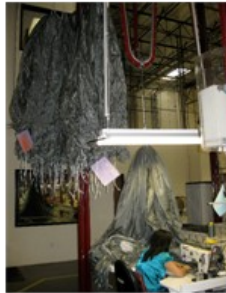
ASNA's unique rail system used to move canopies to the next station of assembly
