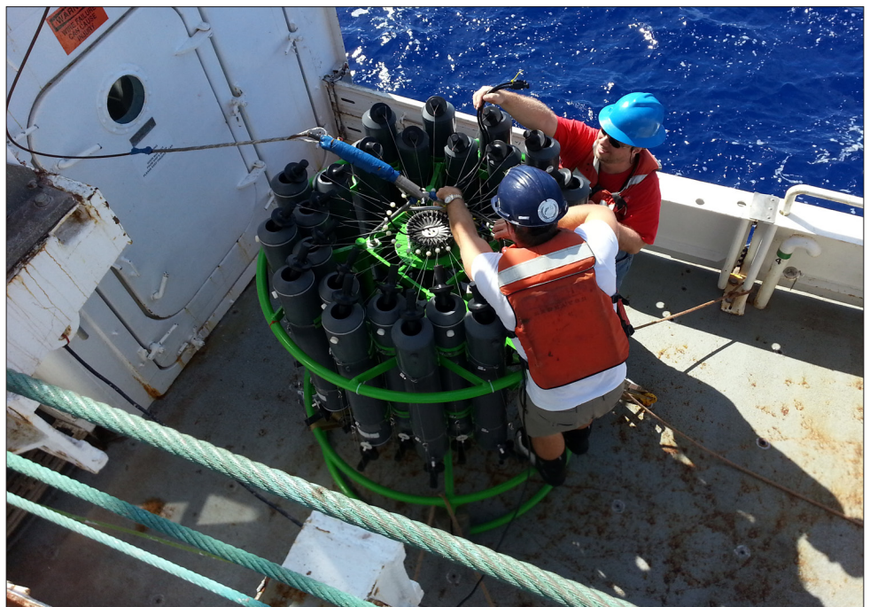
A conductivity-temperature-depth (CTD) instrument is prepared for deployment from aboard the RV Endeavor .
