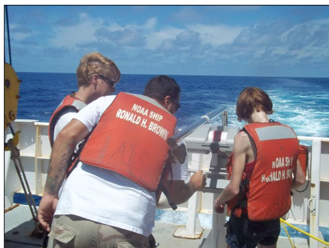
Rick Lumpkin, Grant Rawson, and Verena Hormann of AOML's Physical Oceanography Division prepare the UCTD system for deployment off the stern of the NOAA Ship Ronald H. Brown during the 2011 PIRATA Northeast Extension cruise.
