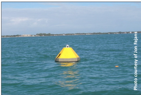
The newly deployed MAP-CO 2 buoy at Cheeca Rocks in the Florida Keys measures carbon dioxide in the atmosphere and ocean.
