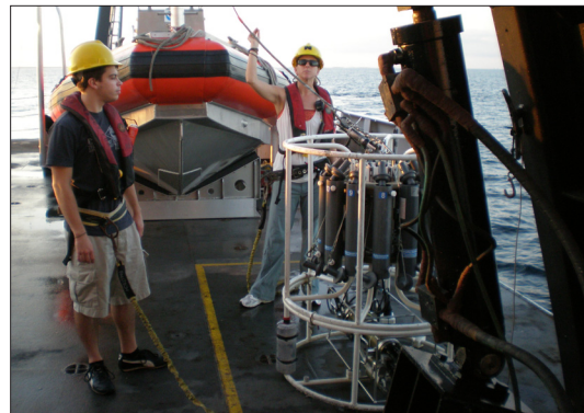
Jakub Bartkowiak of AOML's Environmental Microbiology Laboratory (left) assists with the deployment of a conductivity-temperature-depth (CTD) cast from aboard the NOAA Ship Nancy Foster .
