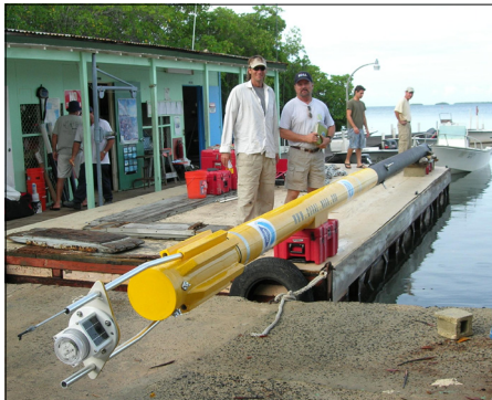
Jeff Absten and Jules Craynock with the new Integrated Coral Observing Network (ICON) station before deployment in La Parguera Marine Reserve, Puerto Rico.
