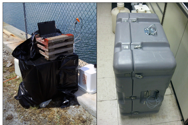
The recording devices for a new ammonia analyzer developed at AOML were originally wrapped in black plastic bags, as shown above on the left at Lake Mabel. However, marauding iguanas necessitated the development of a more defensive-oriented outer packaging for the instrument, as shown in the photograph on the right.
