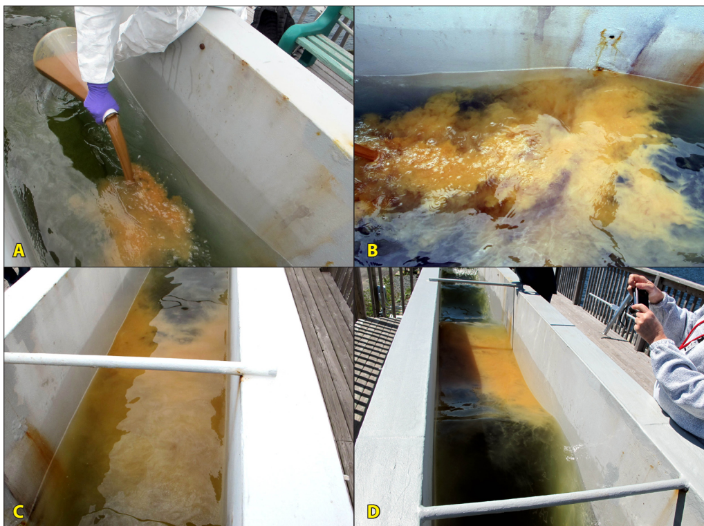
A) Seawater containing MC-252 source oil from the 2010 Gulf of Mexico Deepwater Horizon spill and dispersant is poured into the wave tank at the Center for Offshore Oil and Gas Environmental Research in Nova Scotia, Canada. B) Initial oil front. C) Oil distributes throughout the wave tank. D) A wave generator helps to transport and mix the oil in the tank.
