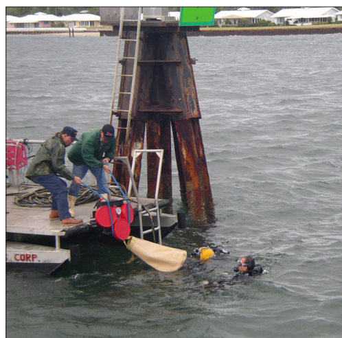
Jules Craynock of AOML (left), along with diving staff, carefully lower "Armando," a horizontal acoustic Doppler profiler, into the Port Everglades Inlet to monitor current flow.
