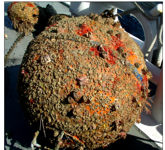
Marine growth that formed on an instrument mooring prevented acoustic release mechanisms from functioning, leaving the mooring stranded on the ocean floor for a year.
