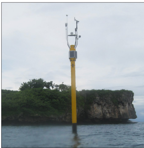
The new, fully instrumented Coral Reef Early Warning System (CREWS) station in Lao Lao Bay, Saipan.
