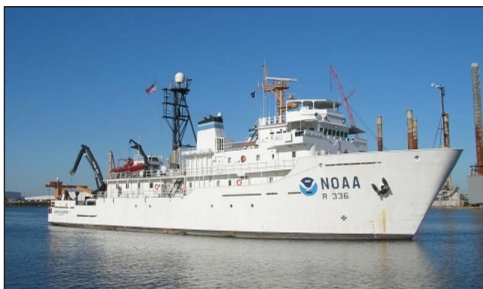
The NOAA Ship Gordon Gunter was the first vessel in the NOAA fleet to use the SEAS AutoIMET system for gathering oceanographic and meteorological data.
