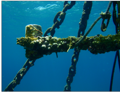
Barnacles and other marine growth are visible on the support chains that anchor the St. Croix station to the ocean floor, as well as on one of the subsurface instruments.
