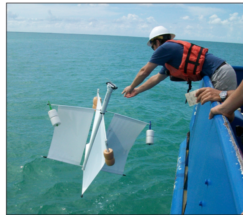
Three satellite-tracked surface drifting buoys were deployed to monitor ocean currents and provide sea surface temperature data.
