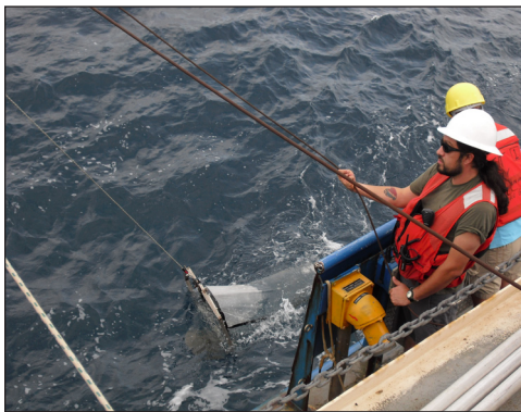
Neuston net tows enabled researchers to gather ichthyoplankton samples and tar balls along the western Florida shelf.
