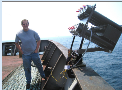
Kyle Seaton of PhOD on the stern of the Horizon Navigator , next to a mounted XBT auto-launcher.
