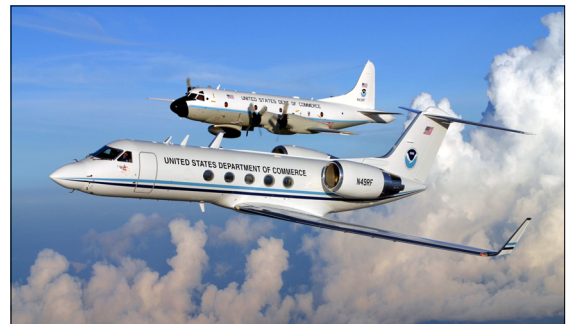
NOAA's Gulfstream-IV jet (foreground) and WP-3D Orion turboprop (background) "hurricane hunter" aircraft are critical to HRD's annual field program. These specially-instrumented airborne observing platforms gather data from the inner core of tropical cyclones and their surrounding environment.
