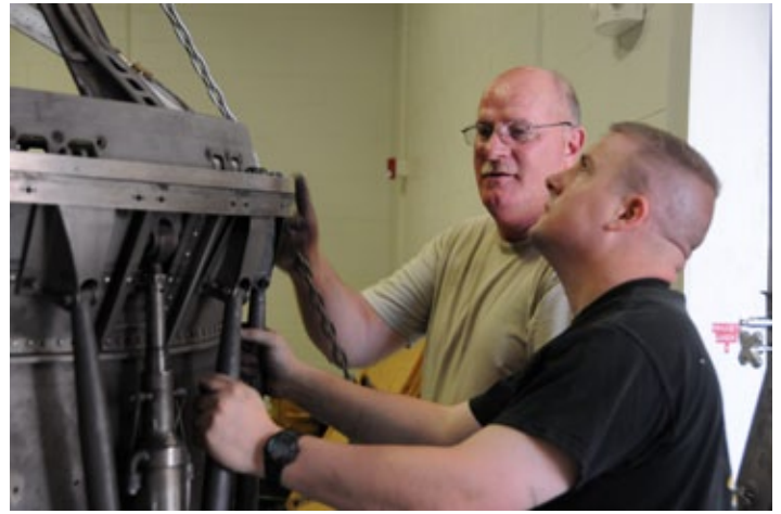
Master Sgt. Tony Bowmaker and Tech. Sgt. Jayme Gabbard assemble B-1 engines which will be installed in the B-1 displayed in the air park.
