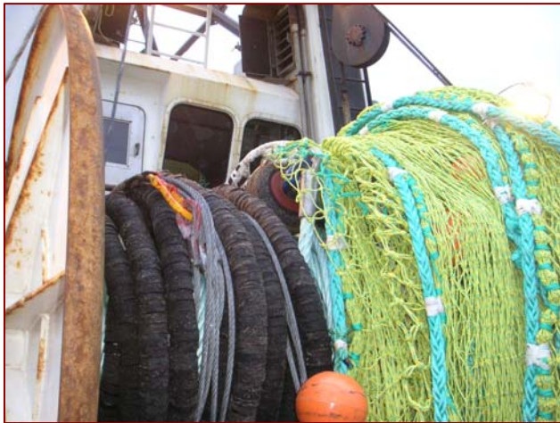
Footrope, net and sweeps wrapped on forward net reel, one bobbin showing in upper center
