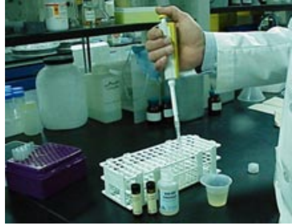
Photo 19. Adding zero calibrator, control, and sample extracts to tubes.
