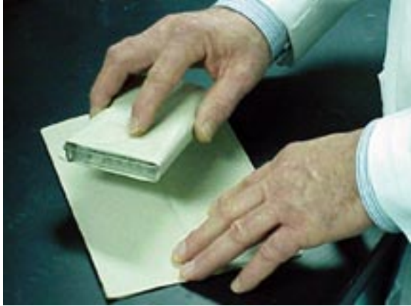
Photo 12. Removing water droplets from wells.
