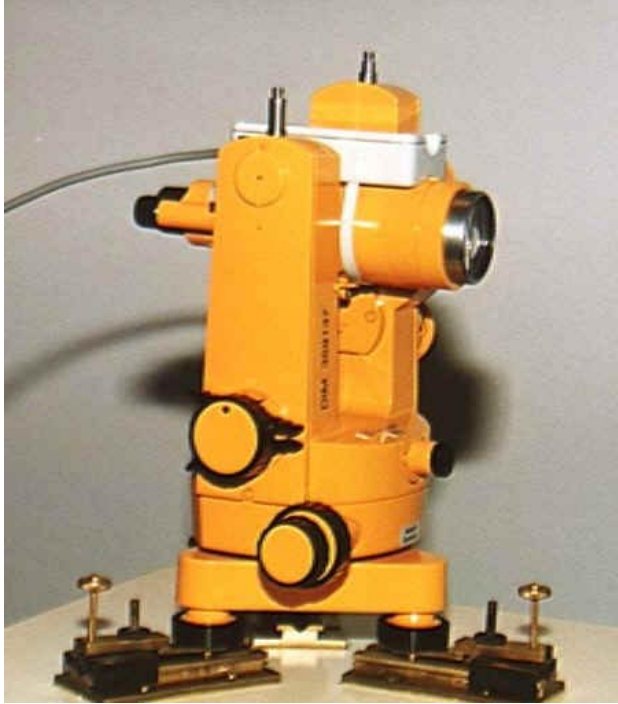
Fig. 5. A declination-inclination magnetometer of the type used to measure the absolute magnetic field direction.
