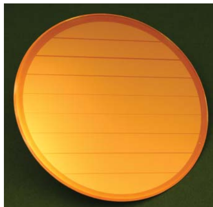
Figure 2. Processed substrate with various bridge widths defined.
