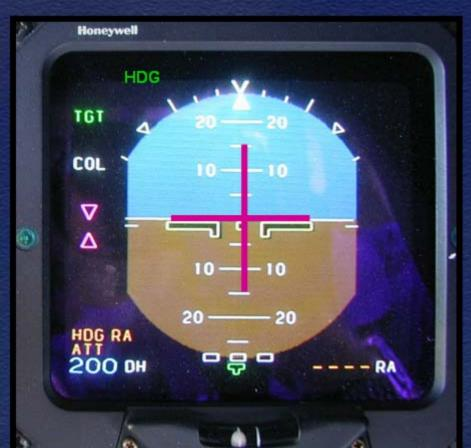
Ensure that all operators of helicopters equipped with either the SPZ-7000 or SPZ-7600 dual digital automatic flight control systems provide training that includes information on flight director and coupling status annunciations; the command cue presentations when only the pitch or the roll mode is engaged; and, if applicable, the differences between the SPZ-7000 and the SPZ-7600. (A-06-20)
