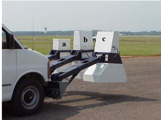
Figure 4. Three impulse GPR antennas mounted on the front bumper of a typical test vehicle: (a) 1 GHz center frequency, (b) 500 MHz center frequency, (c) 250 MHz center frequency.
