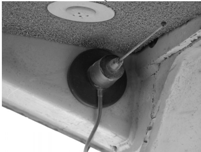
Radio Antenna in Cab.
