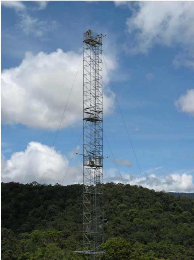
Figure 2: A view on the main 70 m tall flux tower at BFS (left) and one of the two additional towers for measuring horizontal advection (right) Photos H. Kreilein.
