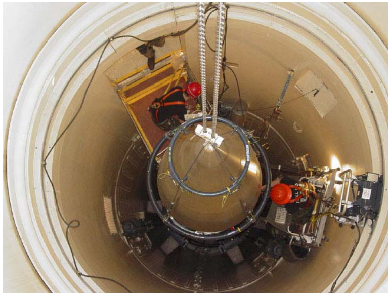
An Air Force Space Command crew removes the nose section of a Minuteman III missile in a silo at Malmstrom AFB, Montana, early in 2003. Portions of the missile were to undergo flight testing in a launch from Vandenberg AFB as part of Air Force Space Command's continuing evaluation program for the remaining inventory of ICBMs. (Photograph courtesy Air Force Space Command News Service)
