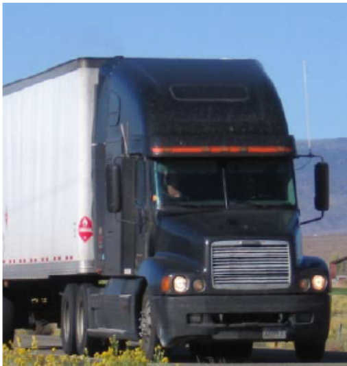
Aerodynamic styled truck with low profile front, aerodynamic bumper, full-height roof fairing, hidden exhaust stacks, and fuel tank side fairings.
