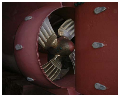
Figure 3.11 Nozzles Enclosing Propeller to Reduce Friction Losses
