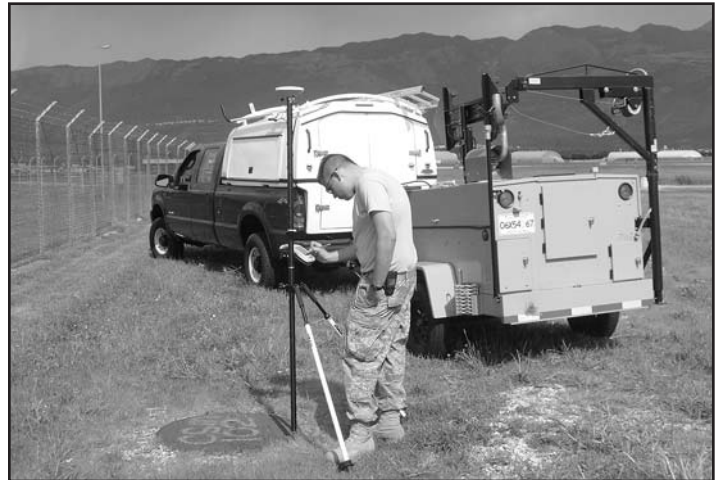
Staff Sgt. Pat Hickmann records data from the Trimble survey equipment while at Aviano AB, Italy. (Photo submitted by Lt. Col. James Loux)
