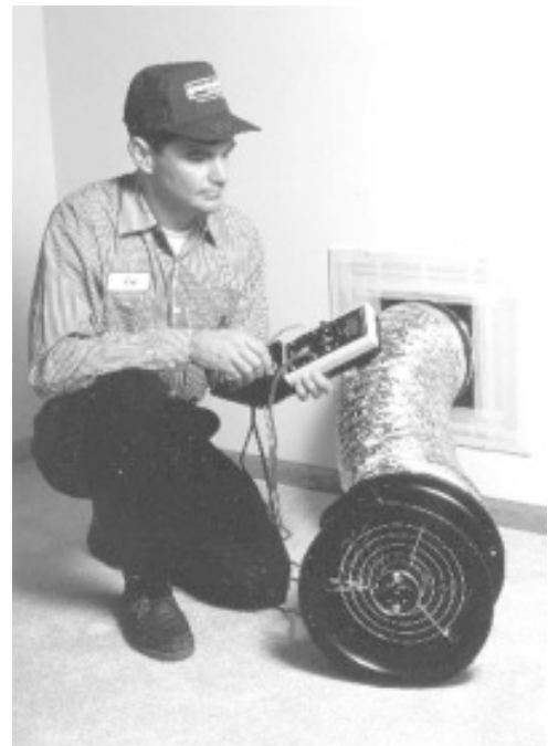
Duct Blower —Used to measure duct leakage. (Courtesy of The Energy Conservatory)
