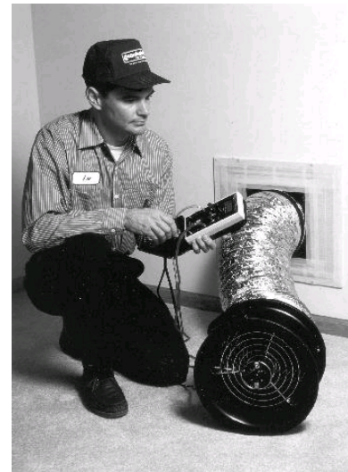
The Duct Blower—Used to measure duct leakage. (Courtesy of The Energy Conservatory)
