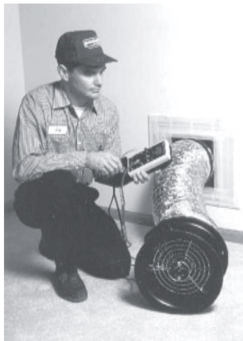
Duct Blower —Used to measure duct leakage. (Courtesy of The Energy Conservatory)
