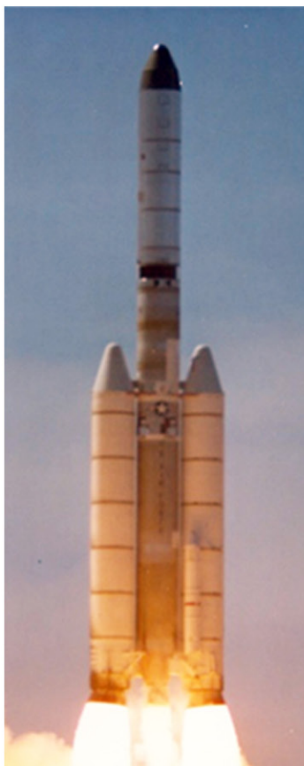
Launch of Hexagon Mission 1215 on 3/16/1979, using a Titan III D booster with 5-segment solid rockets.
