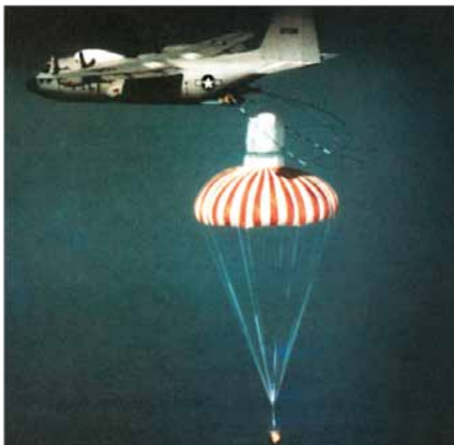
Figure 3. Aerial Recovery of Hexagon Film by JC-130 Aircraft (Reprinted from Oder, et. al., 1992, p. 98).
