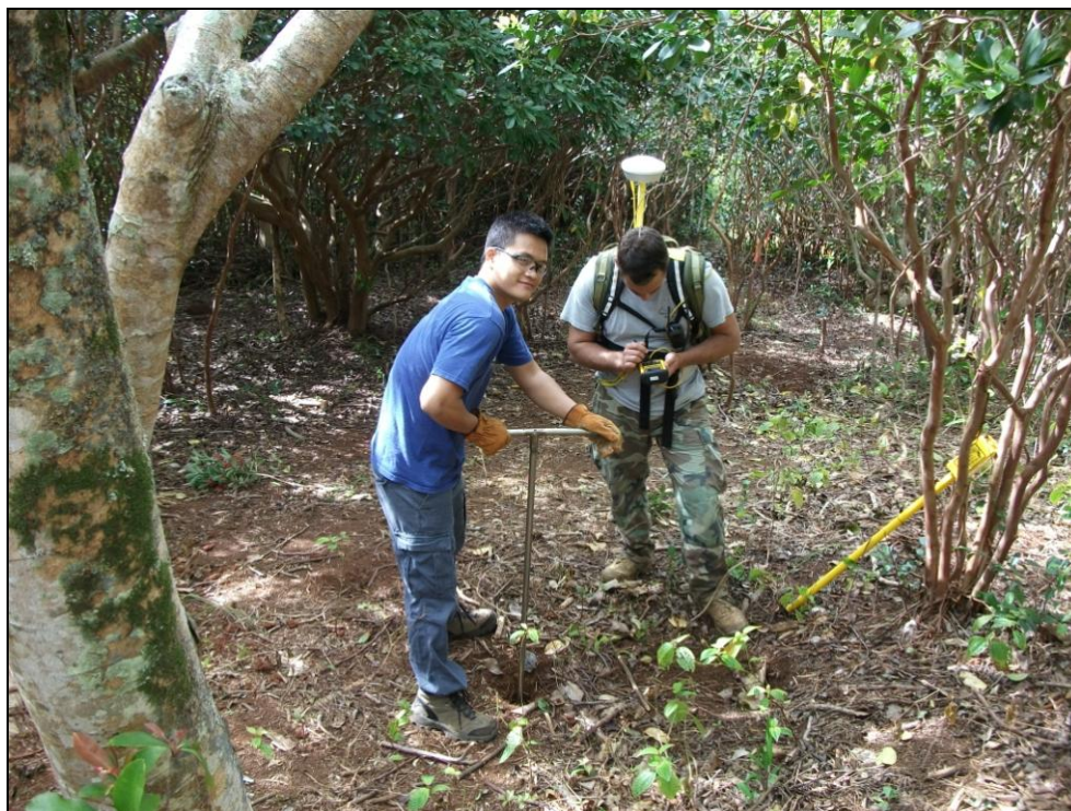
Photo 18 Subsurface Soil Discrete Sampling in AOC-04
