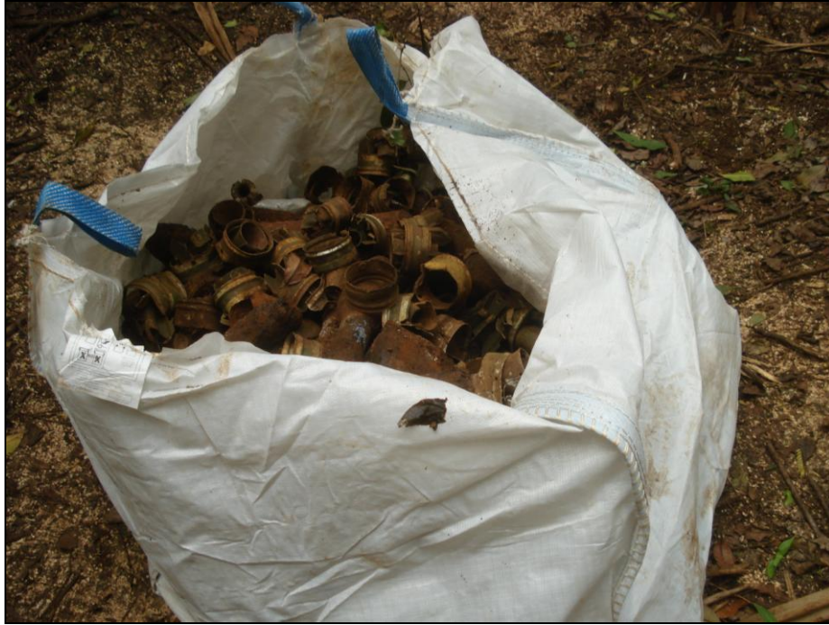
Photo 13 Munitions Debris Preparation for Transportation at Processing Area
