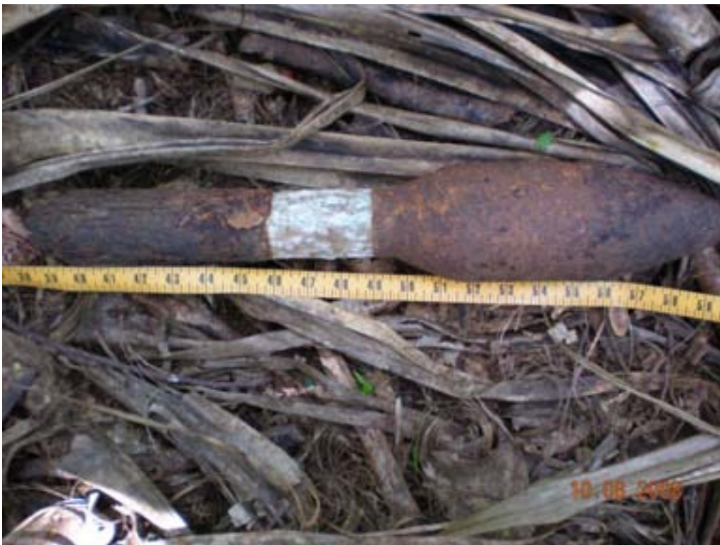
Figure D-8: UXO Item ID 206. Fuzed & Fired 3.5" HEAT Rocket, Fin Missing
