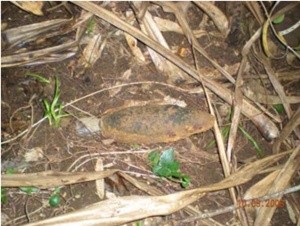
Figure D-7: UXO Item ID 36. Fuzed 3.5" HEAT Rocket Warhead, Motor Buried
