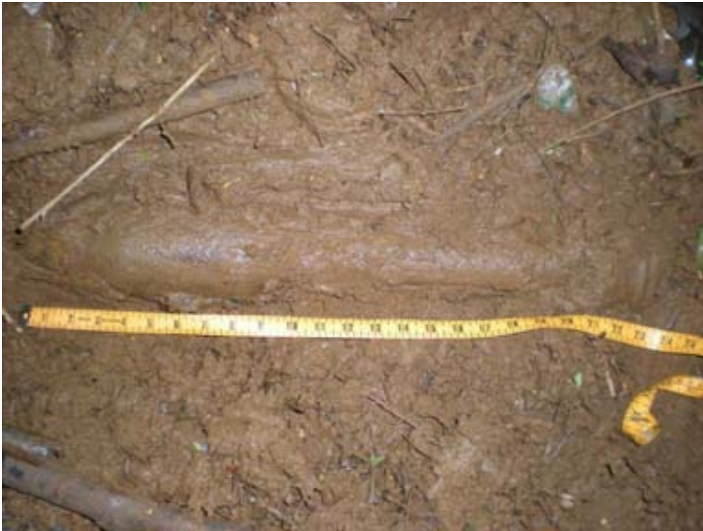
Figure D-6: UXO Item ID 100. Partially Buried Fuzed & Fired 3.5" HEAT Rocket
