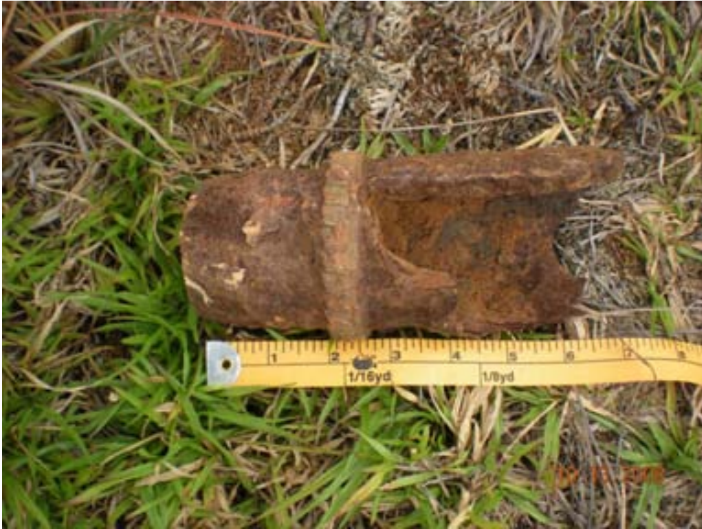
Figure D-11: Base Section Fragment, 75mm HE Projectile, Empty/Inert
