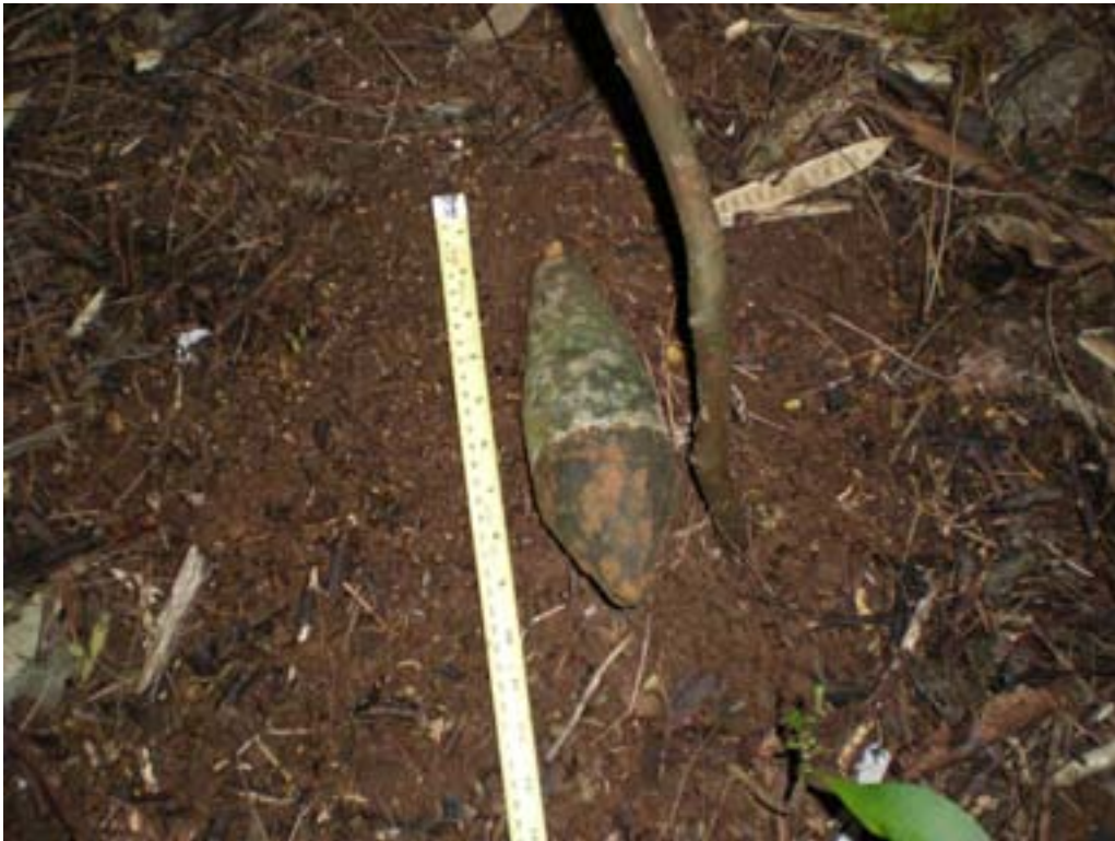
Figure D-17: MD Item ID 130. M29 Practice Rifle Grenade Warhead
