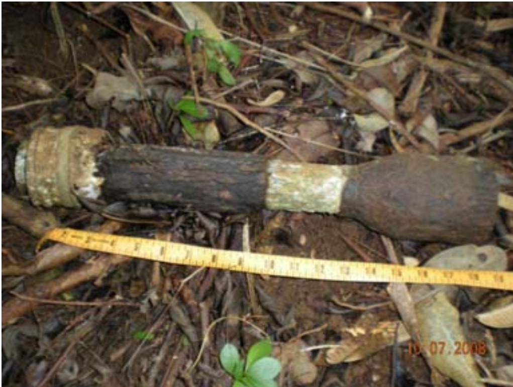
Figure D-9: MD Item ID 3. Practice 3.5" Anti-Tank Rocket, Fired and Inert
