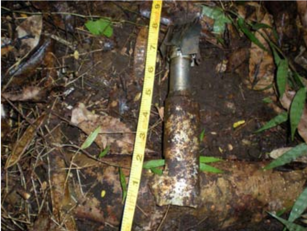
Figure D-13: M127 Series Hand Signal Flare, Expanded/Inert
