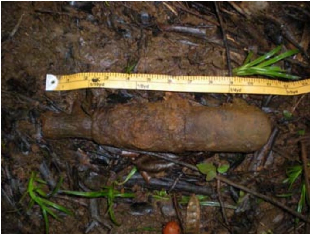
Figure D-12: UXO Item ID 219. Fired & Fuzed 2.36" HEAT Rocket Warhead
