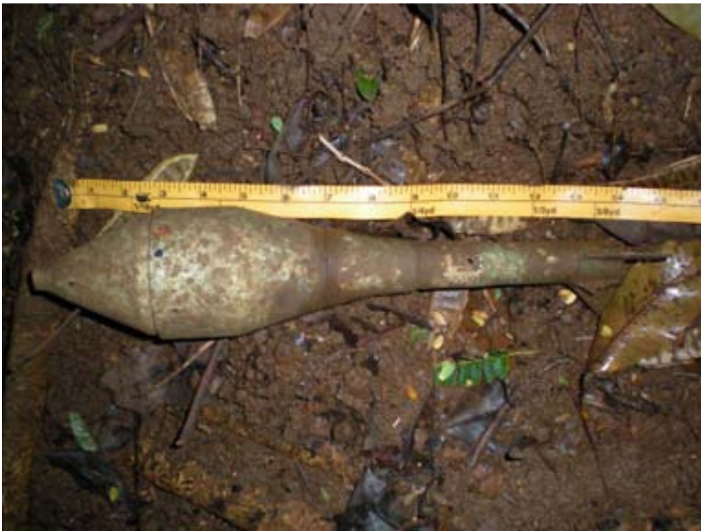
Figure D-14: UXO Item ID 310. M28 HEAT Rifle Grenade, Nose Fuze Broken Off
