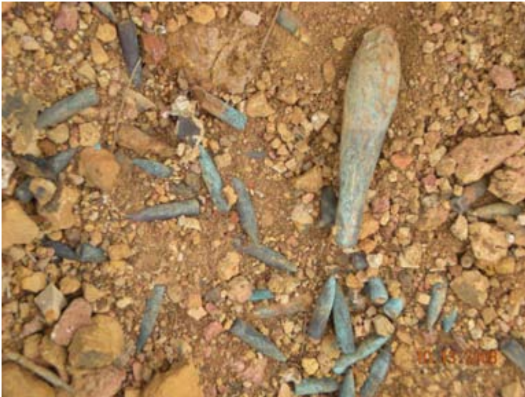
Figure D-20: Cell 22, Copper Slug from 3.5" HEAT Rocket Warhead
