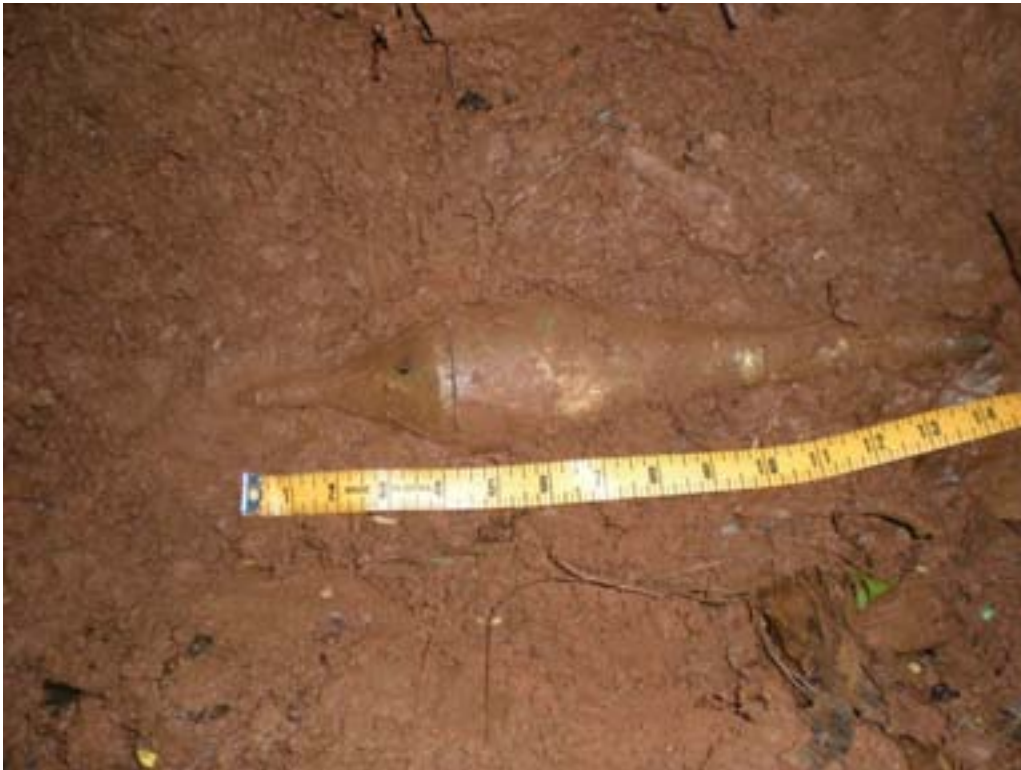
Figure D-15: UXO Item ID 351. M28 HEAT Rifle Grenade, Fuzed
