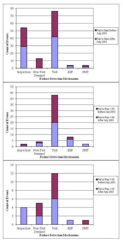
Figure 21. TDP component failure distribution by period, failure mode, and method of detection.
