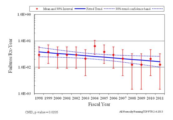
Figure 18. Frequency (events per reactor year) of FTR events, normally running TDPs.
