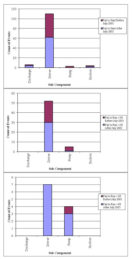
Figure 19. TDP failure breakdown by period, sub component, and failure mode.
