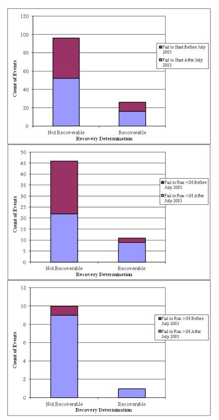
Figure 22. TDP component failure distribution by period, failure mode, and recovery.
