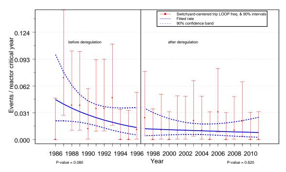
Figure 4. Trend plot of LOOP frequency for 1986–1996 and 1997–2011. Switchyard-centered LOOPs: trend plot of industry performance during critical operation.
