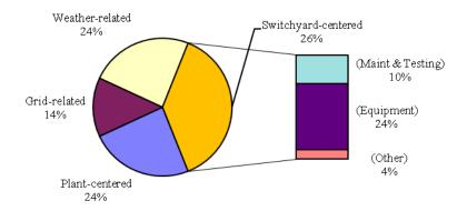
Figure 2. Distribution of LOOP categories (per plant unit) while shutdown (1997 to 2011).
