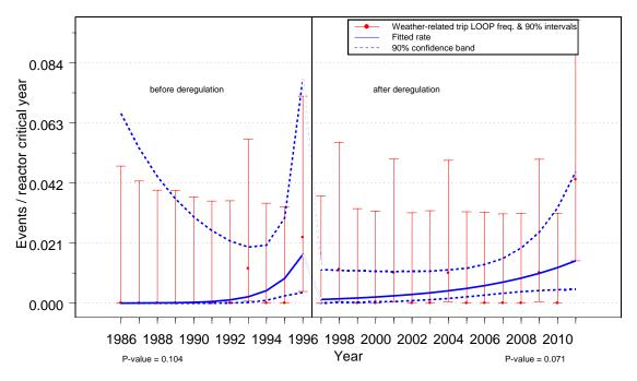
Figure 6. Trend plot of LOOP frequency for 1986–1996 and 1997–2011. Weather-related LOOPs: trend plot of industry performance during critical operation.
