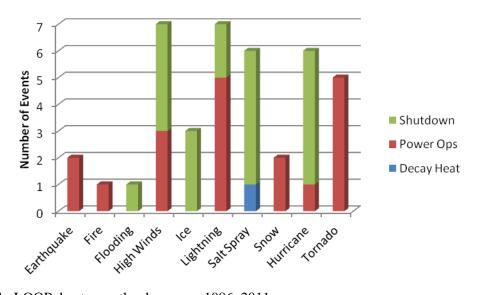
Figure 14. LOOP due to weather by cause, 1986–2011.
