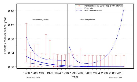
Figure 3. Trend plot of LOOP frequency for 1986–1996 and 1997–2011. Plant-centered LOOPs: trend plot of industry performance during critical operation.
