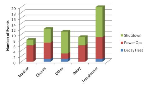
Figure 12. LOOP due to equipment failure by cause, 1986–2011.
