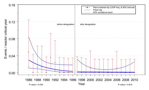
Figure 3. Trend plot of LOOP frequency for 1986–1996 and 1997–2010. Plant-centered LOOPs: trend plot of industry performance during critical operation.
