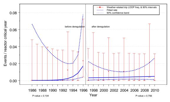
Figure 6. Trend plot of LOOP frequency for 1986–1996 and 1997–2010. Weather-related LOOPs: trend plot of industry performance during critical operation.
