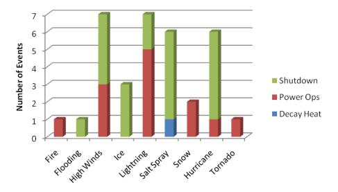
Figure 14. LOOP due to weather by cause, 1986–2010.
