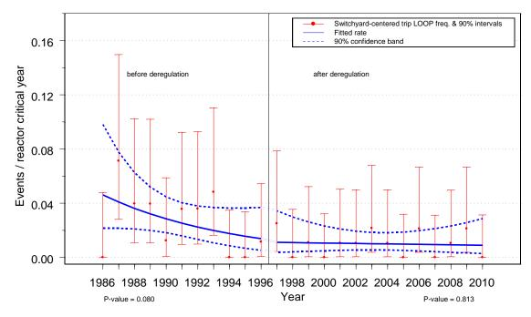
Figure 4. Trend plot of LOOP frequency for 1986–1996 and 1997–2010. Switchyard-centered LOOPs: trend plot of industry performance during critical operation.
