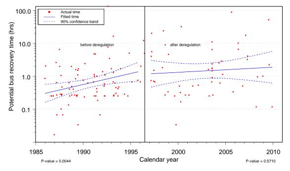
**Note:** The increasing trend over 1986–1996 is statistically significant (p-value for the slope is 0.004), while the slightly increasing trend over 1997–2010 is not statistically significant (p-value for the slope is 0.55).
