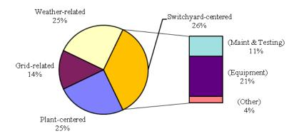
Figure 2. Distribution of LOOP categories (per plant unit) while shutdown (1997 to 2010).
