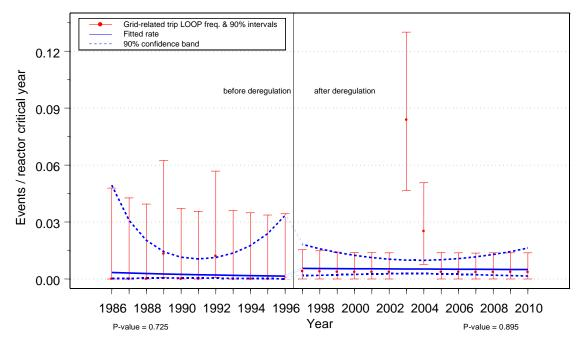
**Note:** The confidence interval for 2003 does not account for the dependence of the events and is, therefore, too narrow (by an undetermined amount).
