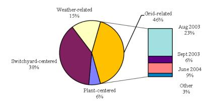
Figure 1. Distribution LOOP categories (per plant unit) during critical operation (1997 to 2010).
