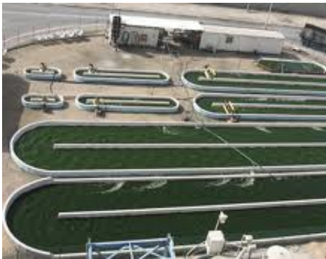
Algal raceways, one method of industrial-scale cultivation of algae
