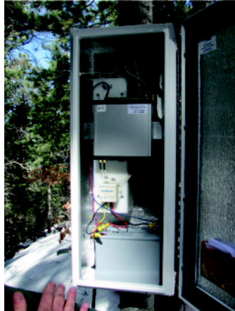
□ Neutron detector installed for field studies in northern New Mexico
