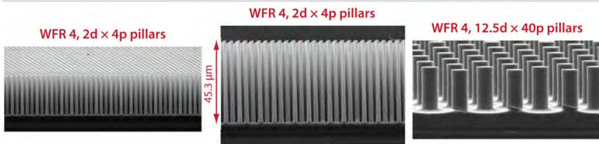
Figure 8. Scanning electron microscope images of Si pillars, showing two different diameters and pitches in the three images
