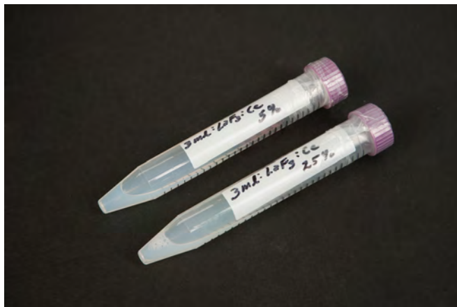
Figure 1. Detector from RMD with 5% LaF 3 :Ce and 25% LaF 3 :Ce nanoparticle loading by mass
