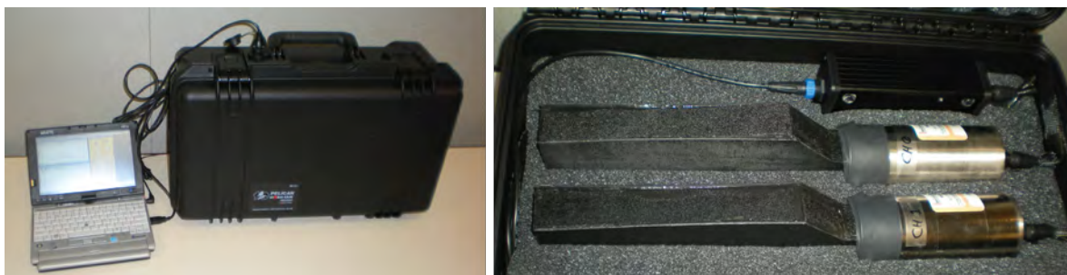
Figure 7. Portable muon counter made with two smaller-size paddles. Paddles were sized to fit within a small pelican case. The Bridgeport Instruments eMorpho TwinBase PMT bases are low power and can be powered by a single USB port on a battery-powered laptop.
