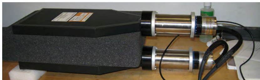
Figure 3. Two large plastic scintillator paddles that make up the muon channel in the fixed neutron-muon observatory
