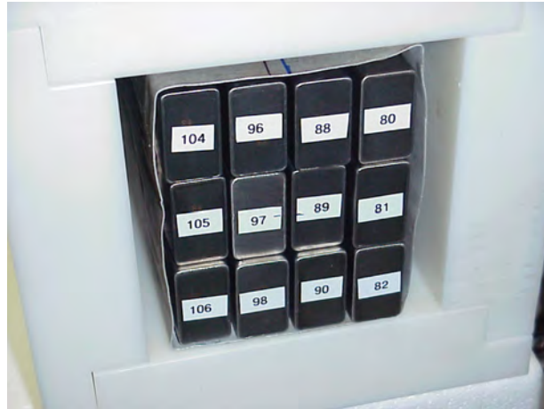
Figure 1. The 4 \times 3 array of 2.5 \times 3.8 cm ^3\text{He} tubes used in the experiments, viewed end on. The tube array is shielded by 0.1 cm thick Cd and 5 cm thick polyethylene. The numbers on the tube ends are part of the MCNP input data.
