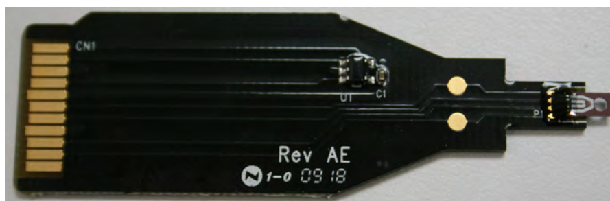
Figure 2. Fully assembled microcantilever with a standard SD connector
