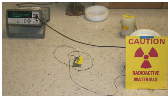
Figure 3. Experimental neutron setup. The ^{252}\text{Cf} source was placed outside of the HDPE enclosure. The EPM detectors were placed inside the enclosure. The HDPE functioned as a neutron energy moderator.
