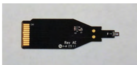
Figure 1. PMC die (far right) attached to a plastic circuit board for plug-in to a standard mini-SD connector
