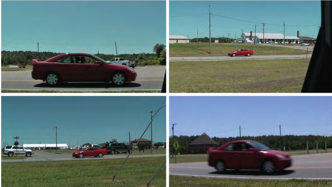
Figure 5. Sample images, test site #2, four camera views at 1:00 p.m. This figure illustrates the foreshortening of the vehicle due to aspect angle and the variation in apparent vehicle size due to distance to the vehicle. The images in the top left and bottom right illustrate smearing variation due to shutter speed. This type of imagery will allow us to test the robustness of future algorithms.
