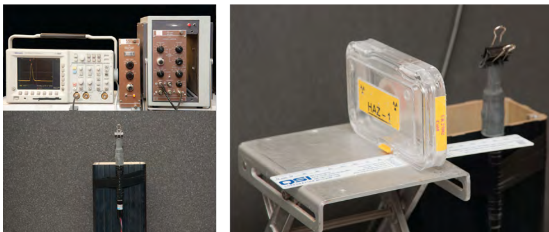
Figure 2. Detector setup for studying the nanocomposite detector. (left) The oscilloscope, power supply, and electronics are shown in the upper part of the photo, while the (liquid) detector assembly is shown below, resting on top of the photomultiplier tube, wrapped in black tape to make the assembly light tight. Signal and high-voltage cables are connected to the detector. (right) The detector assembly is to the right of the 60 Co source.
