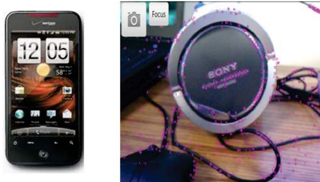
Figure 4. (left) Android phone and (right) output of application run on Android phone. The purple dots are overlaid on the image captured by the phone and represent the output of this OpenCV edge algorithm.
