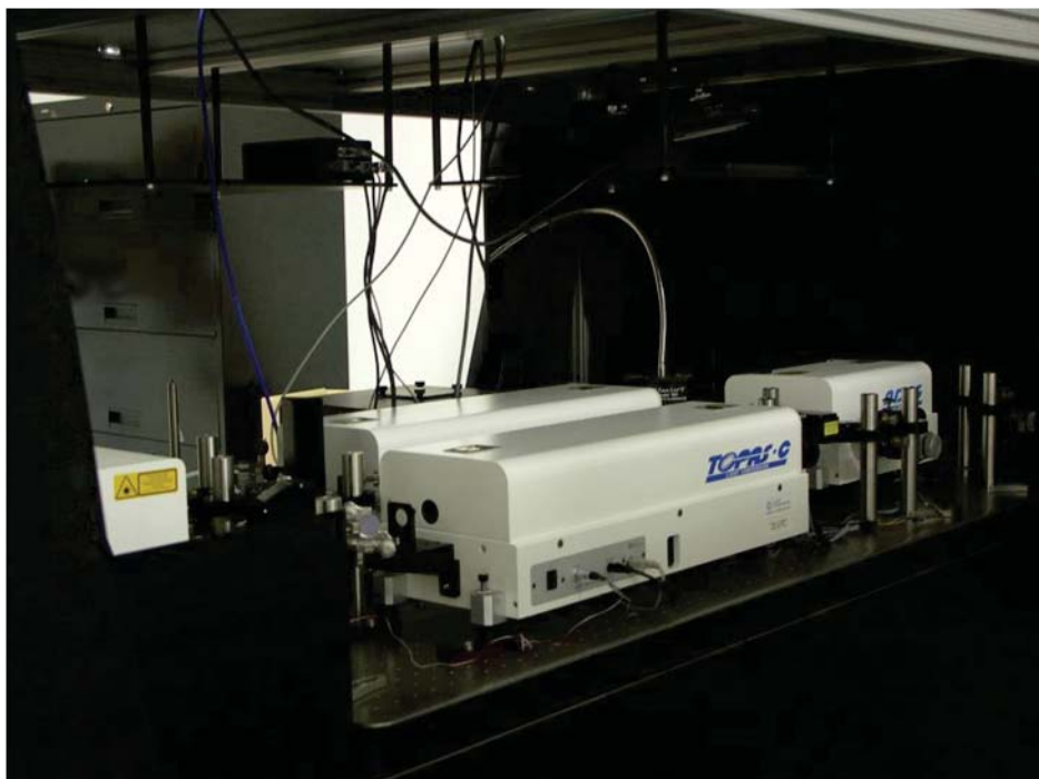
Figure 7. The TOPAS-C system as installed at Livermore Operations. Shown are the TOPAS-C, the mixer stage, the deep ultraviolet module, the delay line, and a corner of the pump laser.
