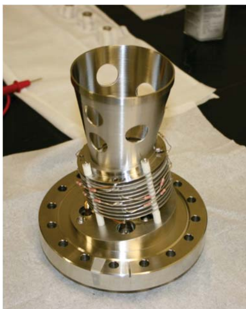
Figure 3. Mini-TOF reflectron assembly with the ion shield mounted to the entrance electrode of the device. The resistor bridge is shown along the outside of the lens stack. Holes were cut into the ion shield so that background gases could be efficiently evacuated during pump down. A nickel mesh (not shown) was placed over the holes using a conduct epoxy.
