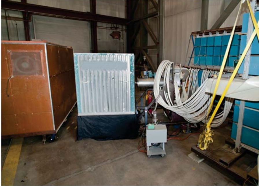
Figure 2. An aircraft shipping container being interrogated using the DPF. The shipping container is in the center, the detector enclosed inside a Faraday cage is on the left, and the DPF assembly is on the right.
