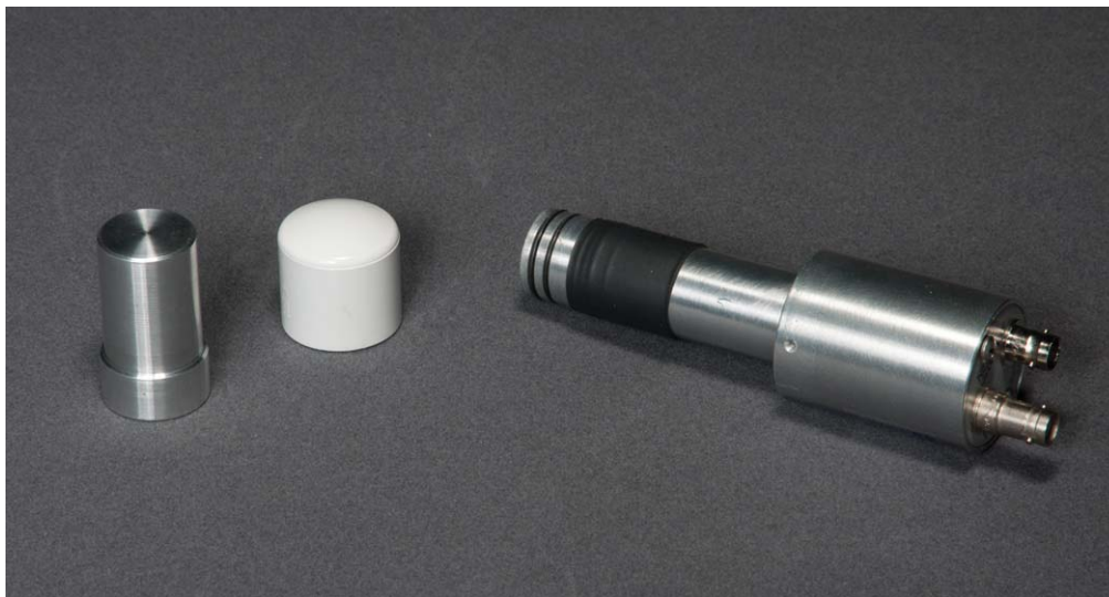
Figure 2. A light-tight mount was made up of the (left) aluminum detector mount, (middle) outer protective cap, and (right) PMT
