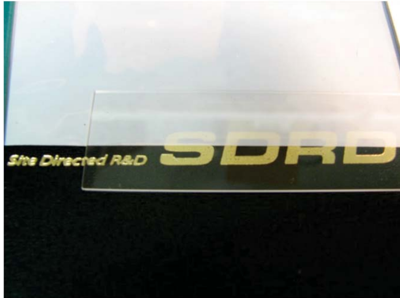
Figure 2. Opalux thin film on clear plastic substrate placed over colored text on black background. Note high opacity.
