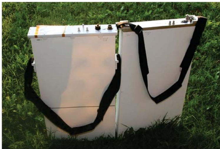
Figure 1. Two-panel NMC. The left panel has 100 straws and the right one has 60 straws. Each panel’s external dimension is 70 × 39 × 6.25 cm and the combined weight is 29.4 kg (64.8 lb).
