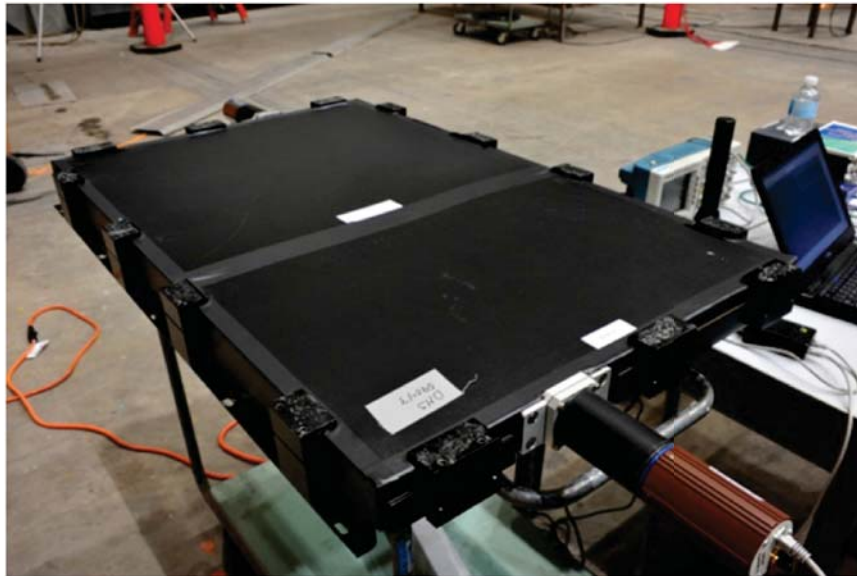
Figure 1. A view of one of the PVT detectors used on this project with two ORTEC digiBASE-E digital gamma spectrometers used for data acquisition
