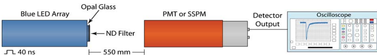
Figure 4. LED array positioned in front of sample detector. The LED array was a 1-inch-square area of surface-mount LEDs. Opal glass diffused the output of the LED array. Pulsed signals were measured on each detector.
