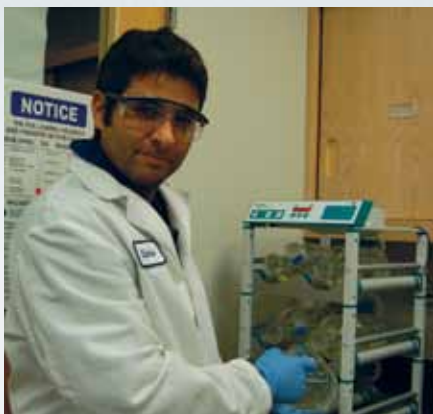
Principal investigator Mayali with the “rolling bottle” laboratory setup where isotope-labeled marine particles are incubated with bacteria under different climate conditions.
