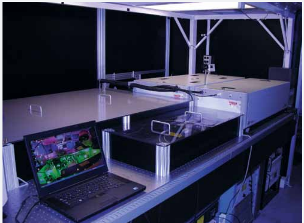
The titanium-doped sapphire inverse free-electron laser drive produces 500-mJ, 100-fs, 785-nm pulses at a 10-Hz repetition rate with a tabletop footprint.
