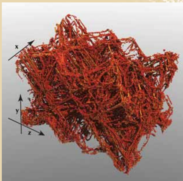
A snapshot of defects in a molecular dynamics simulation of the effects of strain rate on microstructure during dynamic compression. Letters indicate the axes of the three-dimensional simulation space.
