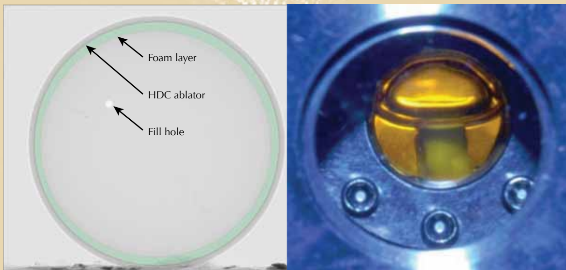
An x-ray radiograph of a 2-mm diameter, 30- \mu\text{m} -thick diamond shell with an approximately 50- \mu\text{m} layer of dicyclopentadiene polymer gel is shown (left), and a 30-mg/cm 3 dicyclopentadiene polymer foam that survived wetting with cryogenic hydrogen (right).
