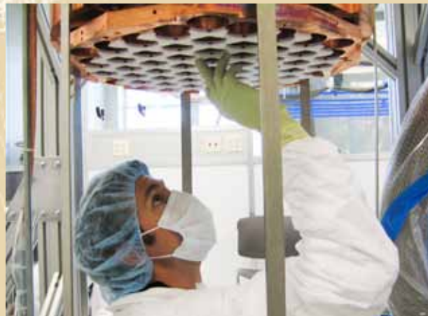
Livermore postdoctoral researcher and collaborator Peter Sorensen installs mounting fixtures for photomultiplier tubes in the Large Underground Xenon Dark Matter Experiment detector.
