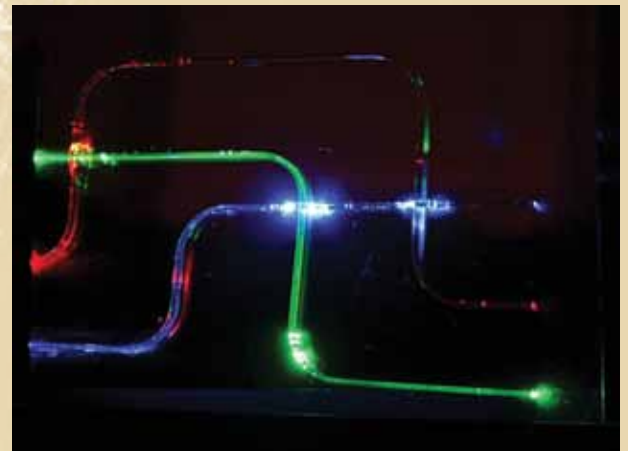
An optical image showing light confinement in three polymer waveguides fabricated with our direct ink writing technique.
