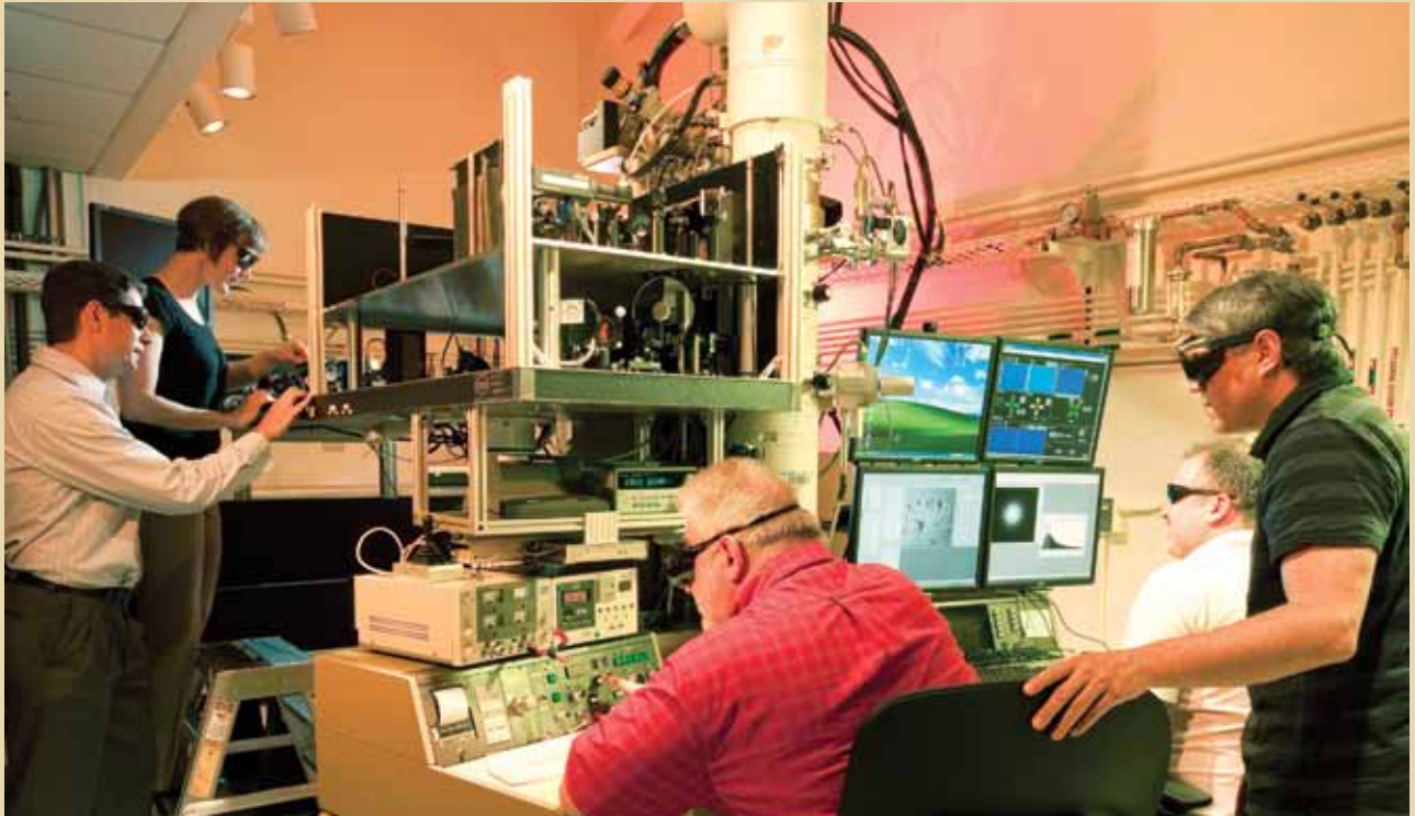
The dynamic transmission electron microscope has already produced new levels of scientific understanding of nanostructure growth, phase transformations, and chemical reactions.
