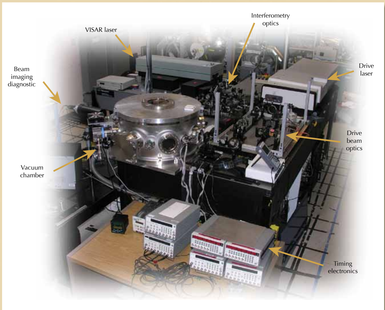
Experimental apparatus at the Laboratory is being used to study shocked foams to validate models of void evolution in materials.
