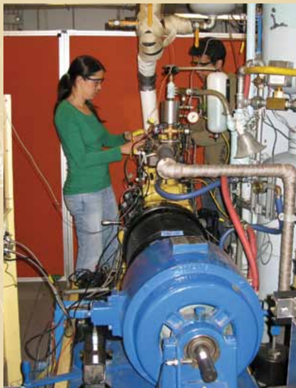
University of California at Berkeley graduate student Vi Rapp (left) and Lawrence Livermore National Laboratory post-doctoral researcher Nick Killingsworth (right) examine the hydrogen–oxygen–argon cooperative fuel research engine.
