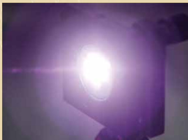
A sub-picosecond laser pulse fired onto a piezoelectric sample produced a compressive shock wave that propagated through the material, generating terahertz radiation.
