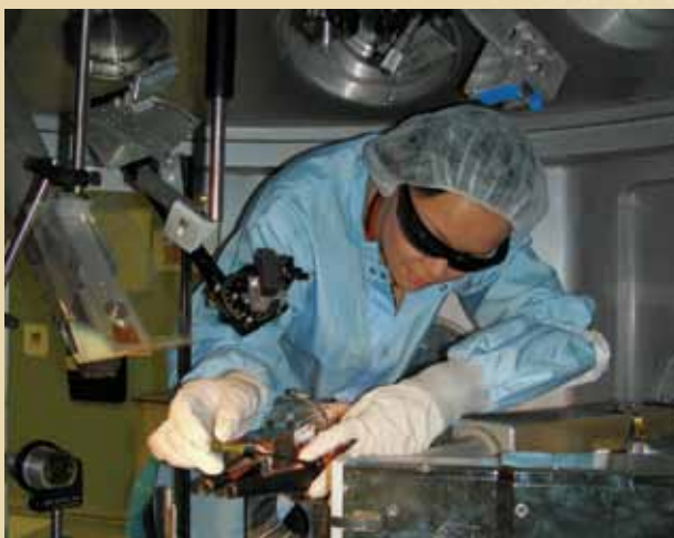
Graduate student Kelly Cone adjusts a soft x-ray spectrometer inside the target chamber of Livermore's petawatt-class Titan laser.
