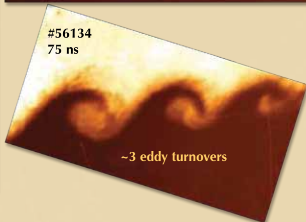
Radiographic images from laser-driven Kelvin–Helmholtz experiments using 100-mg/cm 3 foam, suggesting a transition from a smooth to a more turbulent flow.
