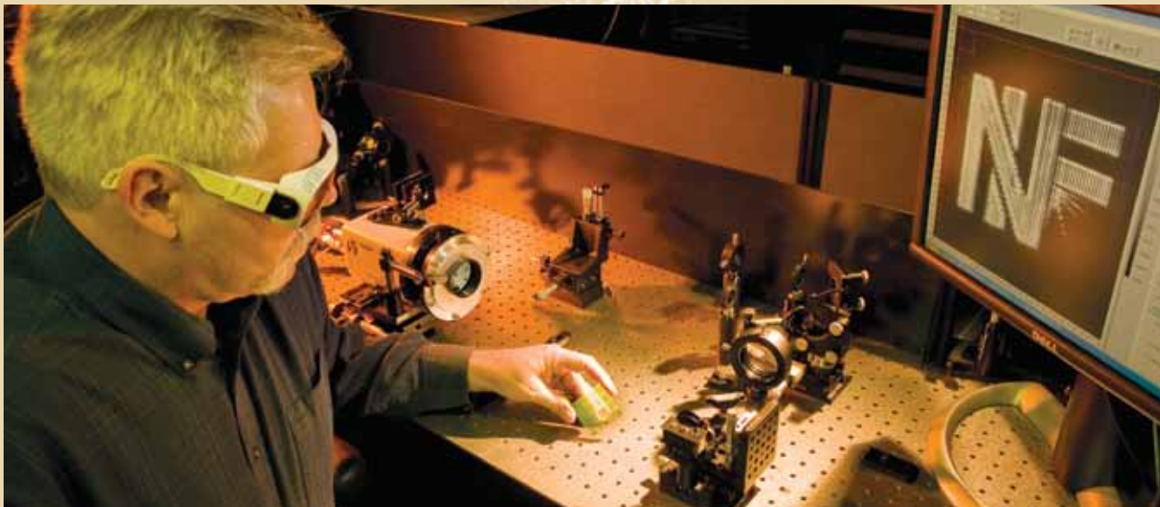
Our LDRD project led to a 2010 R&D 100 award for the grating-actuated transient optical recorder (GATOR), which is designed to acquire sequential images of x rays or optical light in a trillionth of a second or faster during experiments at the National Ignition Facility.
