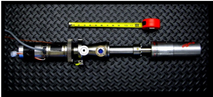
Figure 3. Cryocooler and germanium detector mechanical assembly.
