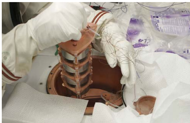
Figure 3. A test string being deployed into the canary cage.
