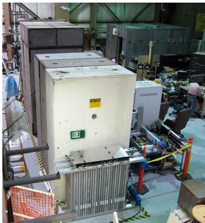
Figure 4. A contour plot (right) showing scattering angle squared at the mid-plane. Next to the plot (left) is a photograph showing the target and the regions of 80-, 40-, and 20-cm thicknesses of lead. The regions are discernible in the reconstruction plot.
