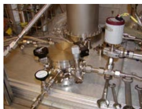
Figure 2. (a) The reaction chamber, shown above, is used to allow UF_6 to react with a humidified atmosphere under controlled temperature and relative humidity. (b) Depending on the amount of moisture present, UF_6 hydrolyses through a number of compounds. All of these intermediates – with the exception of UOF_4 – may coexist.
