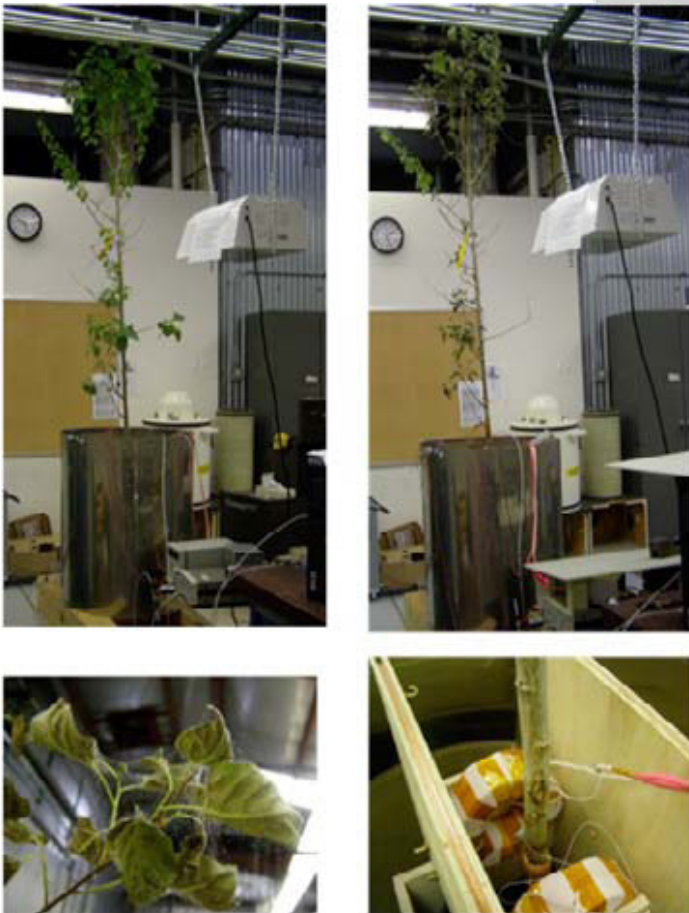
Top row: Two photos of the tree in the ULF NMR system. The NMR system is located inside the silver magnetic shield. The photo at left was taken approximately seven days before the photo at right, and significant decline in leaves is noted. Bottom row: Left shows close up of leaves infected with parasite. Right shows close up of NMR system around tree trunk.
