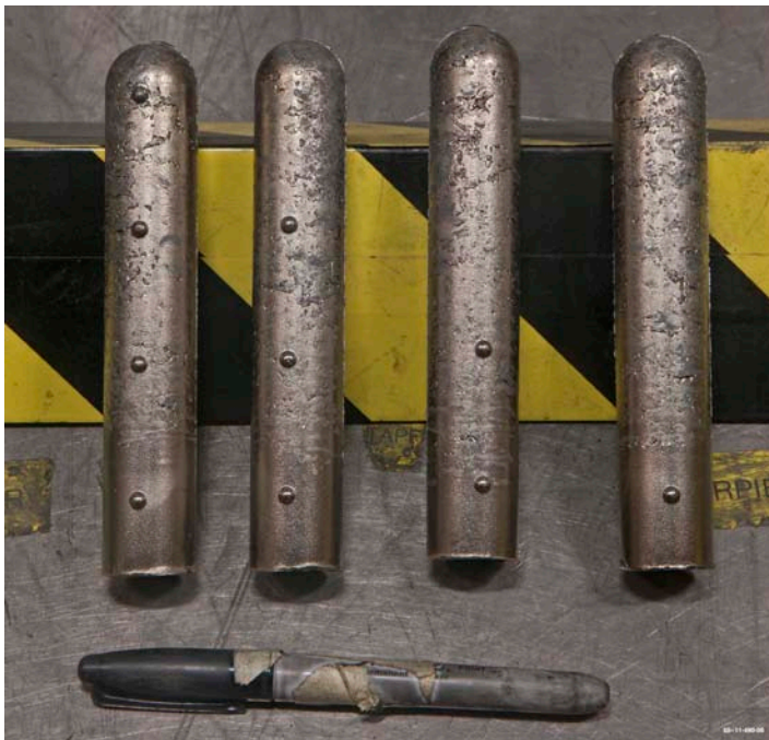
Figure 2. Freshly cast Pu-7 at.% Ga rods, shortly after breaking out of the mold.
