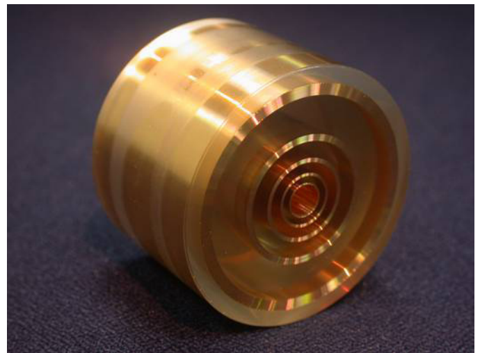
Figure 2. Photograph of the 5 shell multiplier assembly used in the second implosion shot.
