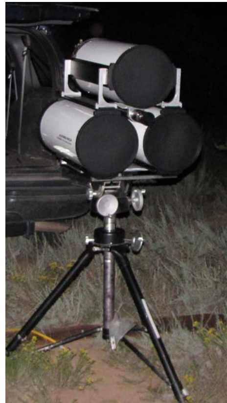
Figure 2. The three 10-inch reflector telescopes (photographed with caps) that collect reflected light in the LIDAR system.
