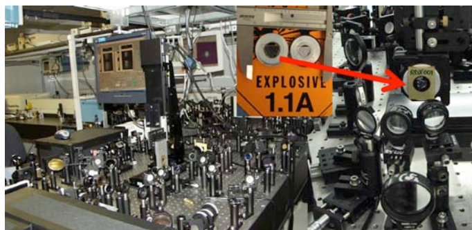
Figure 1. The ultrafast shock experiment allows testing and introduction of numerous diagnostics that allow observation of shock dynamics in explosives, such as the \sim 1 cm RDX crystal shown, on molecular time scales.
