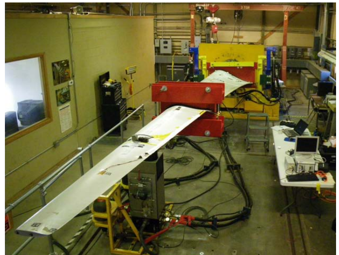
Figure 1. Wind turbine blade during fatigue test.
