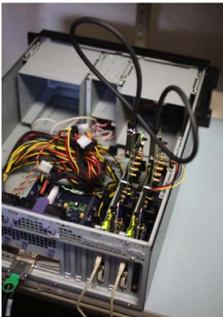
Figure 3. Photograph of compute and network cards in PCI-E slots. This interface allows reconfigurable hardware to efficiently communicate with standard HPC compute nodes.
