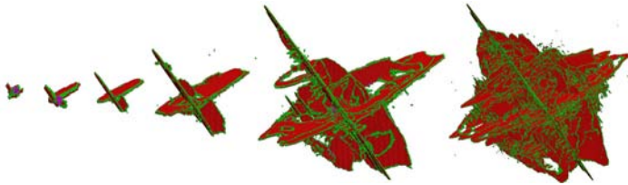
Figure 1. Void growth via dislocation emission studied by a combined accelerated and large-scale MD simulation. An initial 13-atom void in a copper crystal containing 13 thousand atoms is stretched at experimental strain rates using accelerated MD until the first dislocation emission event is detected. At that point, the sample is embedded into a larger (108 million atom) crystal that allows the subsequent processes of dislocation loop emission, growth, and intersection to evolve.
