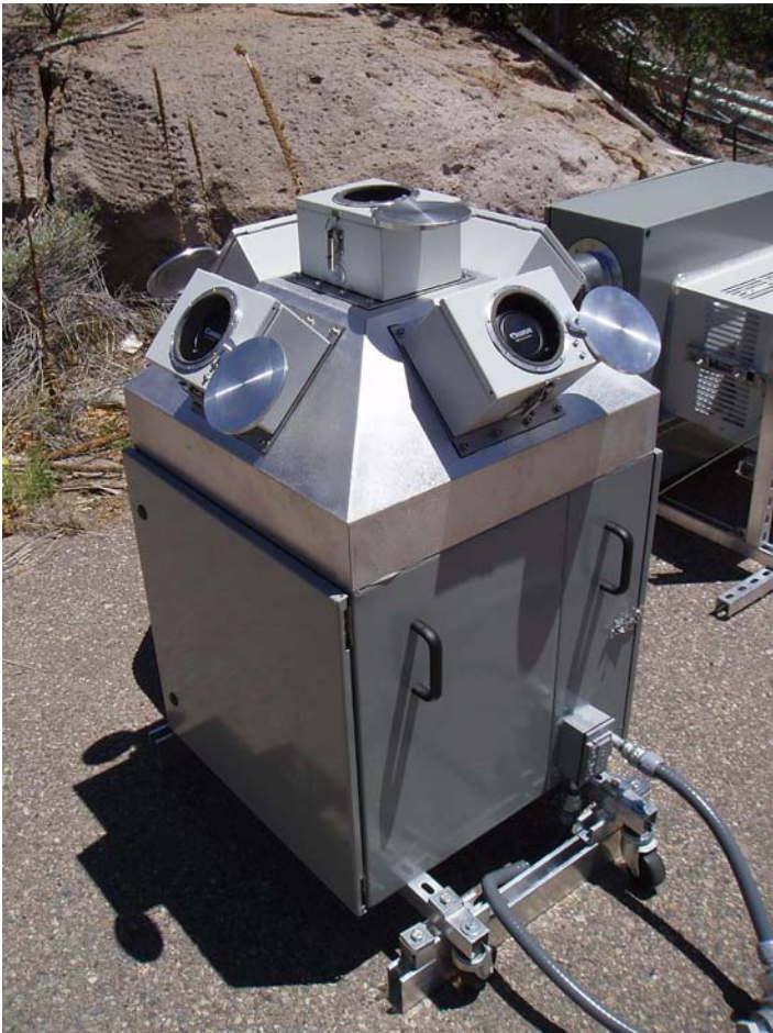
Figure 3. This small observatory called RQD2 (RAPTOR-Q Design 2) is the prototype for nodes in a global network, capable of continuous persistent monitoring of the night sky. The observatory employs five wide field of view imagers that altogether view about 90% of the sky above 14 degrees elevation with the sensitivity of 10th magnitude in 10 seconds.
