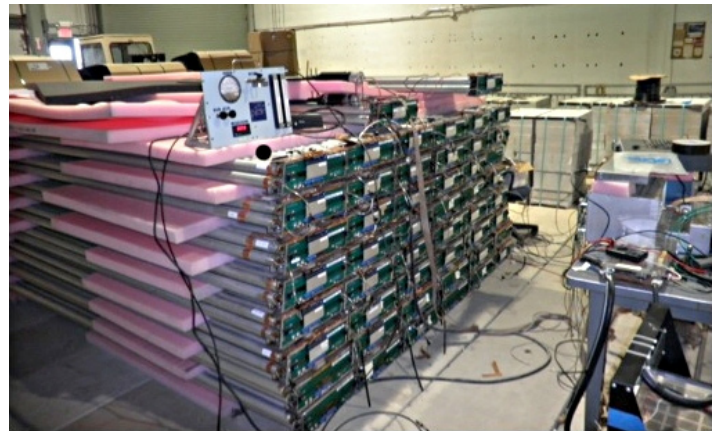
Figure 5. LANL-contributed muon detectors at Fermilab E906 experimental hall for testing and conditioning. Detectors are ready for the final installation.
