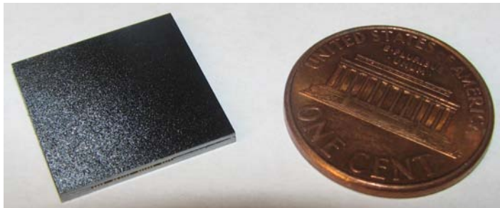
Figure 5. Photograph of the three-channel channel-drop filter and scale.
