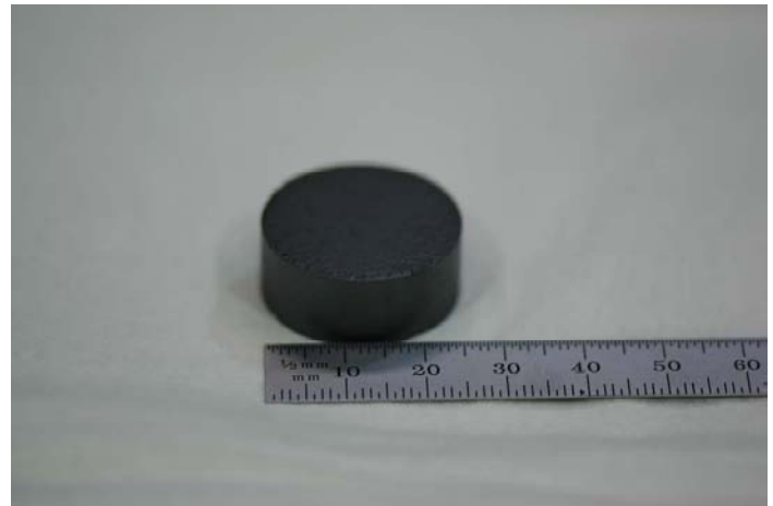
Figure 1. Optical image of depleted \text{UO}_2 pellet.
