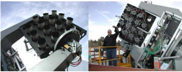
Figure 2. The RAPTOR-K sky monitoring array. This array has the ability to image the full sky every seven minutes down to 16th magnitude using 30 second exposures.
