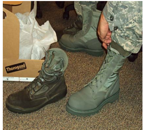
Air Force officials announced the results of the recent ABU combat boot wear test. The boot of choice, which includes a rubber-coated toe and heel, is pictured on the right. Research began to develop a stain-resistant boot to overcome issues with the current suede sage green boot, pictured on the left. (U.S. Air Force photo/Brad Jessmer)
