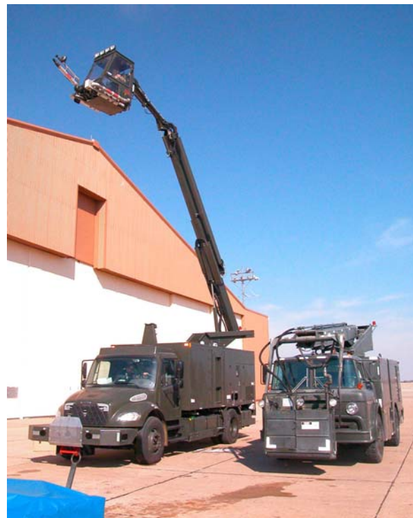
Items like this deicer make the job easier for maintenance members when it comes to taking care of the aircraft and getting it ready to fly during the winter.
